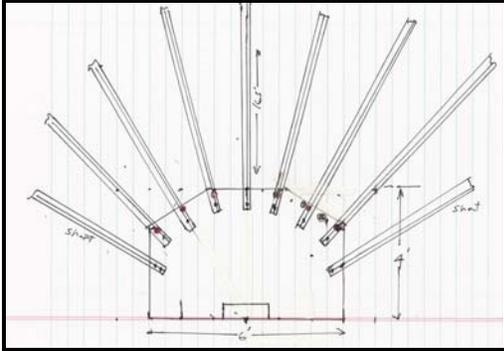
**Fig. 10a - The spokes (6 long and 2 optional short) are attached to a 4' x 6' plywood hub.**
