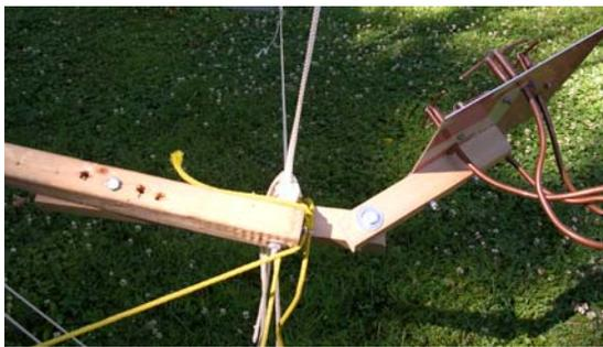
**Fig. 8 - The feed is mounted using several supports to allow optimum positioning**
