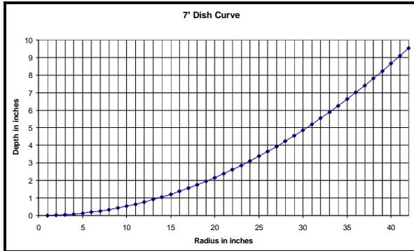
Fig. 2 – Curve of 7' dish with f/d = 0.55.
