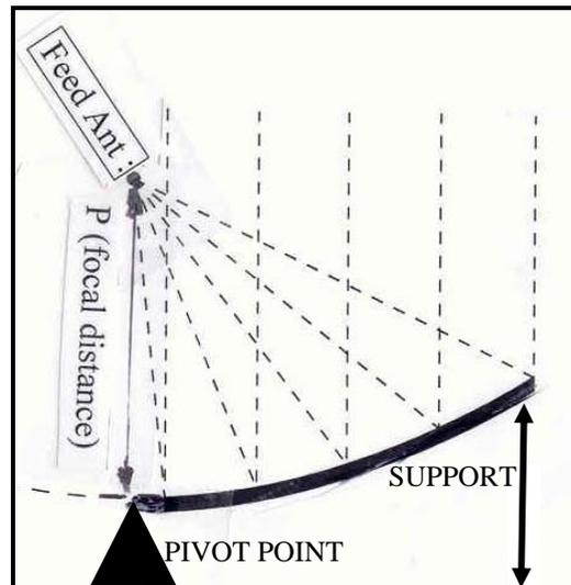
Fig. 4 - The offset dish can be laid on ground (pointing up) when not in use.
