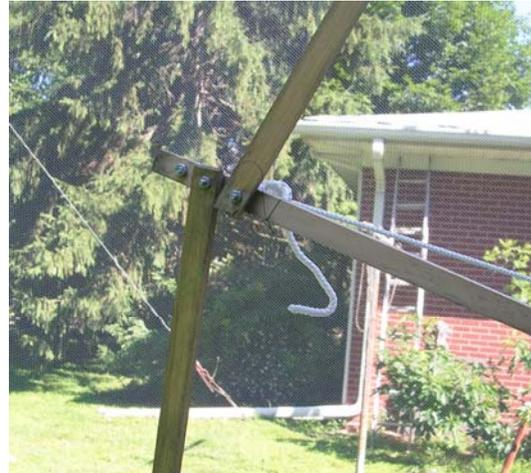
**Fig. 6 - An outside rim is formed from 3.5' lengths of 1/2" x 1/2" modeling strips.**
