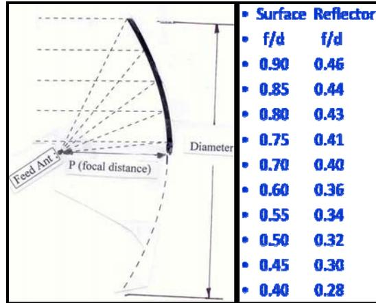
Fig. 3 – a) The feed is located to one side of the reflector, b) Relationship between reflector f/d and equivalent f/d for feed.
