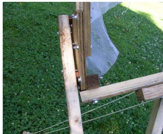
**Fig. 7 - The dish is attached to the feed support by a 2" x 2" block**
